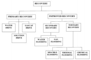
Fig 1.1 Different Methods of Oil Recovery
