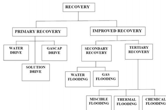
Fig 1.1 Different Methods of Oil Recovery
