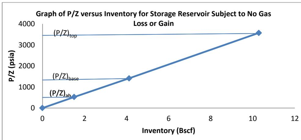
Figure 1  $P/Z$  versus inventory for storage reservoir subject to no gas loss or gain.
