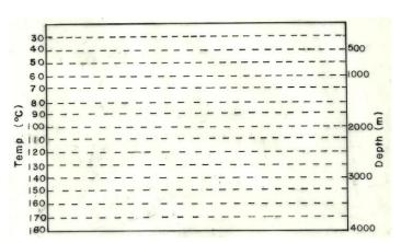
Figure 3. Subsurface temperature grid that assumes a constant surface temperature of  $27^{\circ}C$  and geothermal gradient of  $34^{\circ}C/Km$
