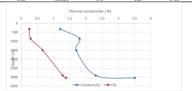
Figure 8. Combined burial and thermal history variation for Kanadi-1 Well, (a) Thermal conductivity/Ro versus Depth
