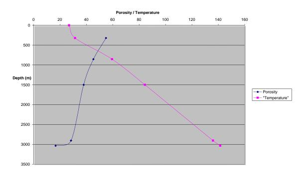
Figure 8. Combined burial and thermal history variation for Kanadi-1 Well, (b) Porosity/Temperature versus depth
