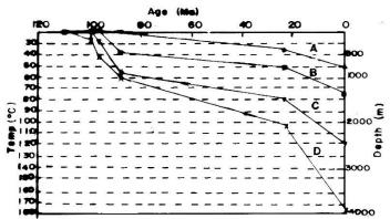
Figure 4. Isomaturity lines on a geological reconstructed model.
