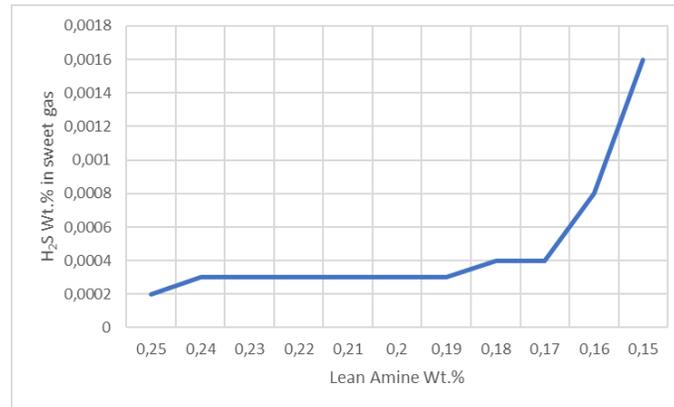
Figure 3. Lean MDEA wt.% versus H<sub>2</sub>S wt. % in sweet gas from absorber
