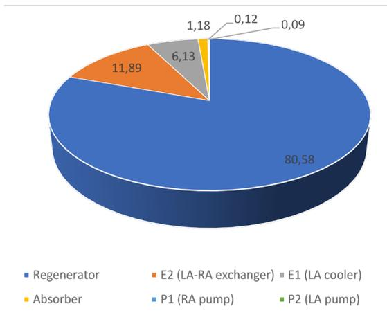
The highest destruction rate is observed in Regenerator with a value of 1937.89 kW and a percentage share of 80.58 % of total destruction, then E2 with a value of 286.05 kW and a percentage share of 11.89 % of total destruction. The percentage share of destruction is shown in Figure. 2. The overall efficiency of exergy is 99.88%.
