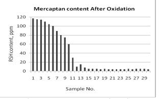
Fig. 5 Light mercaptan content of condensate feed after extraction
