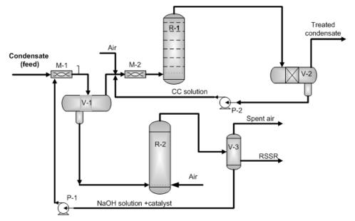
Fig. 1. Simplified PFD of DMC pilot plant
