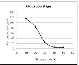
Fig. 3 Temperature effect on oxidation stage reactions
