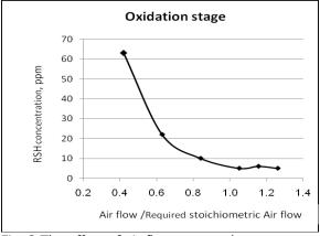
Fig. 2 The effect of air flow rate on demercaptanization in oxidation stage
