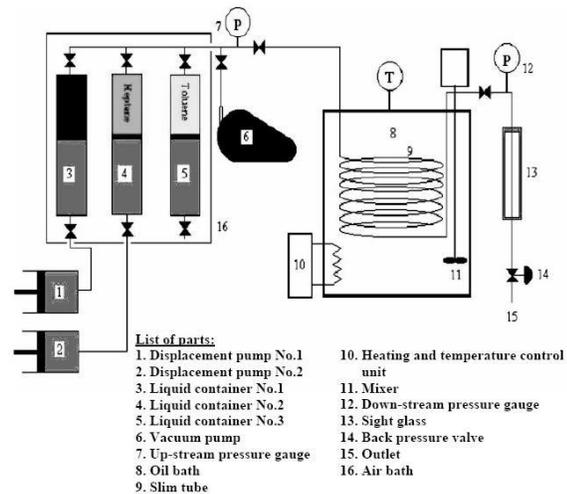
Fig. 4. A schematic diagram of the experimental setup
