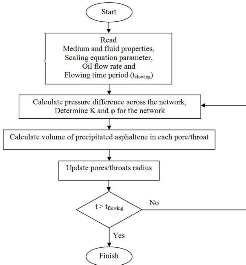
Figure 5. Algorithm for simulation of asphaltene precipitation in network model
