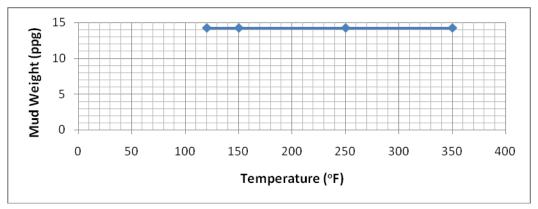
Fig. 8 Effect of aging on mud weight of Versaclean mud
