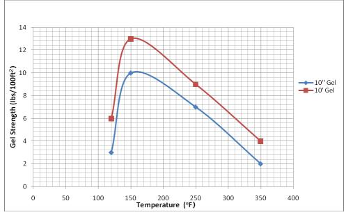
Fig. 5 Effect of aging on gel strength of Versaclean mud
