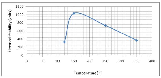
Fig. 6 Effect of aging on electrical stability of Versaclean mud
