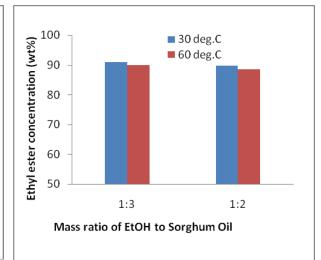
Fig. 4 Effect of reaction temperature on the ethyl ester concentration at  $30^{\circ}$ C and  $60^{\circ}$ C, 1.0% NaOH and 120 minutes
