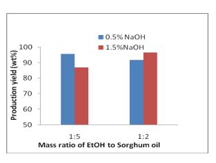
Fig. 1 Effect of mass ratio of ethanol to sorghum oil and catalyst concentration on the production yield at  $30^{\circ}$ C and 120 minutes: 0.5 and 1.5% NaOH
