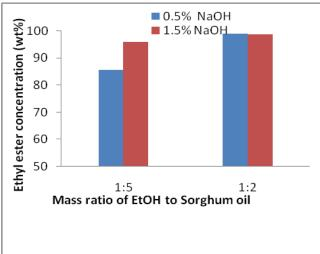
Fig. 2 Effect of mass ratio of ethanol to sorghum oil and catalyst concentration on the ethyl ester concentration at  $30^{\circ}$ C and 120 minutes: 0.5% and 1.5% NaOH.
