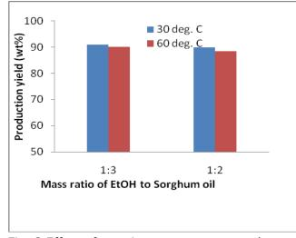
Fig. 3 Effect of reaction temperature on the production yield at 30°C and 60°C, 1.0% NaOH and 120 minutes
