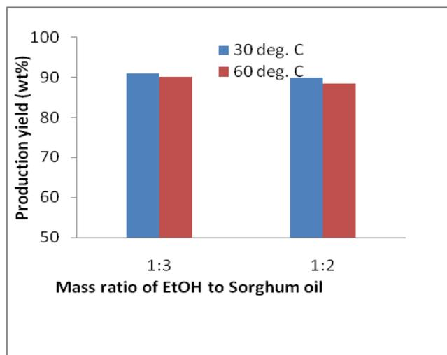
Fig. 3 Effect of reaction temperature on the production yield at 30°C and 60°C, 1.0% NaOH and 120 minutes
