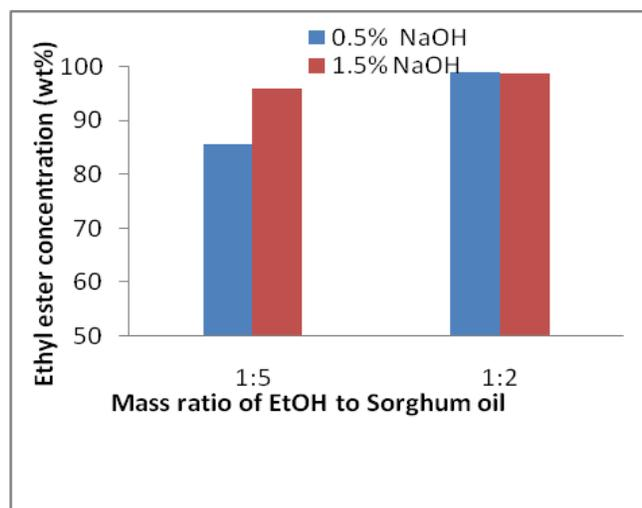
Fig. 2 Effect of mass ratio of ethanol to sorghum oil and catalyst concentration on the ethyl ester concentration at 30°C and 120 minutes: 0.5% and 1.5% NaOH.
