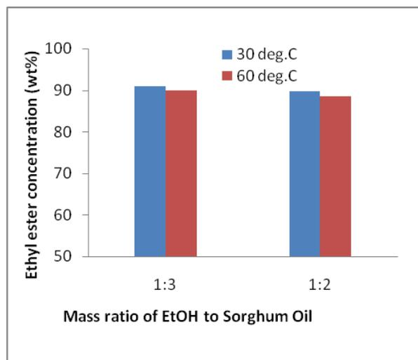
Fig. 4 Effect of reaction temperature on the ethyl ester concentration at 30°C and 60°C, 1.0% NaOH and 120 minutes
