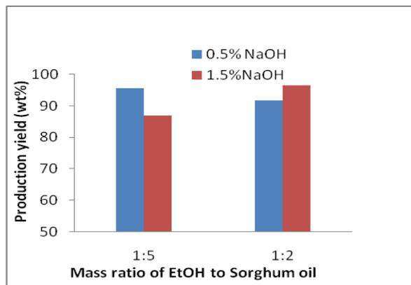
Fig. 1 Effect of mass ratio of ethanol to sorghum oil and catalyst concentration on the production yield at 30°C and 120 minutes: 0.5 and 1.5% NaOH
