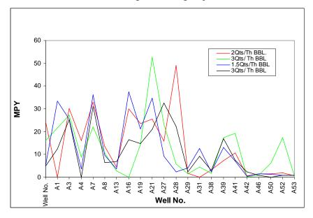
Fig. 5 Inhibitor concentration/corrosion rate
