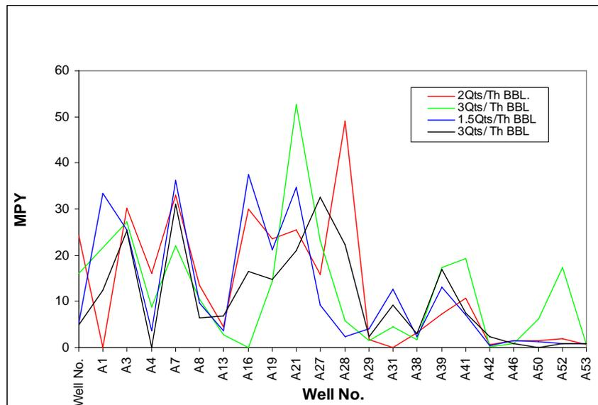
Fig. 5 Inhibitor concentration/corrosion rate
