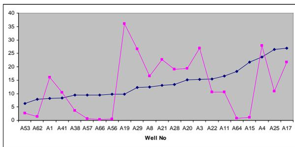
Fig. 4. Relation between corrosion rates and volume of associated gas
