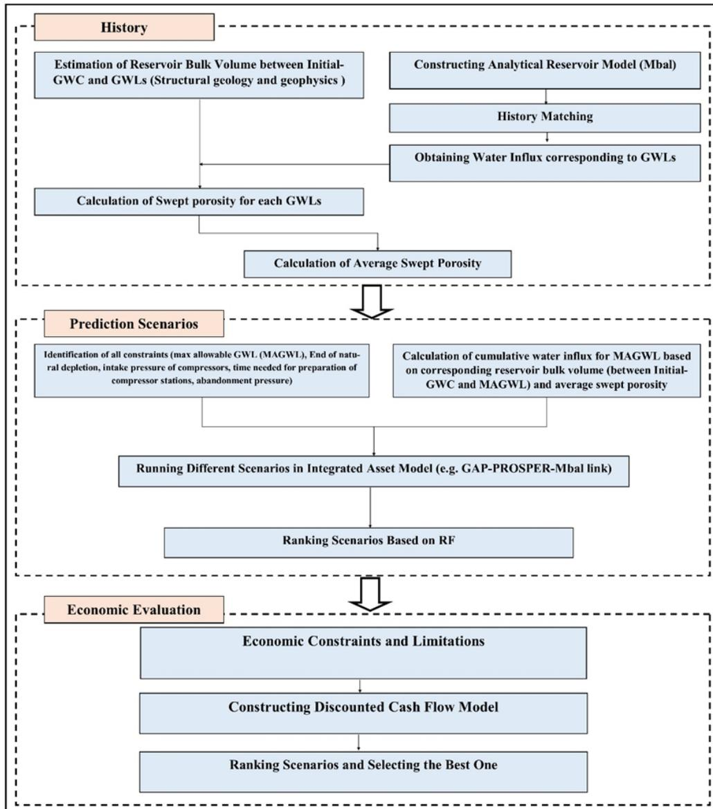
Figure 1. Workflow of evaluation of water rising issue in gas reservoirs
