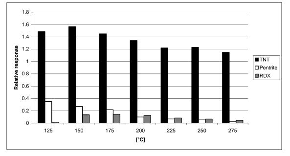
Fig. 1. Average relative response (n=3), calculated to 2,6 DNT, for problematic compounds in the dependence on temperatures of PTV in splitless mode, concentration 10 ng/µl, injected volume 0.5 µl.
