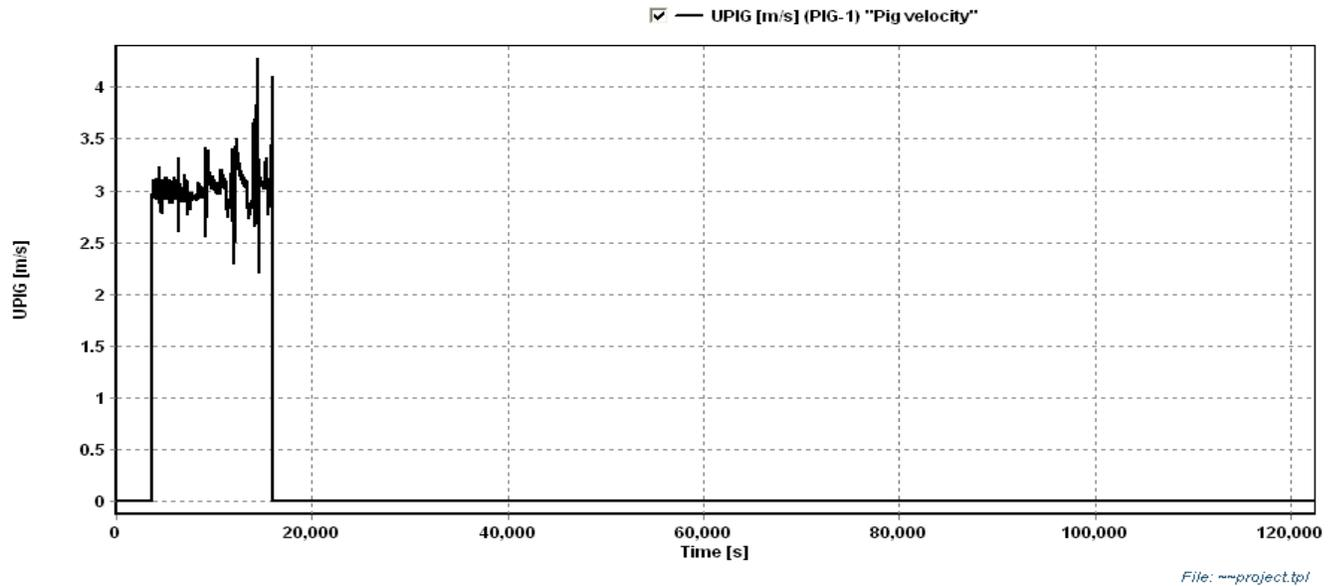
Figure 30. Pig velocity plot to determine the travelling velocity of the pig
