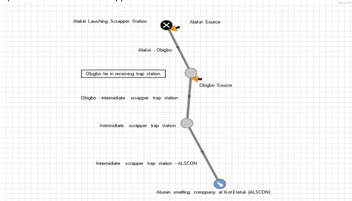
Figure 2. Schematic diagram of OLGA models with nodes and source inlet
