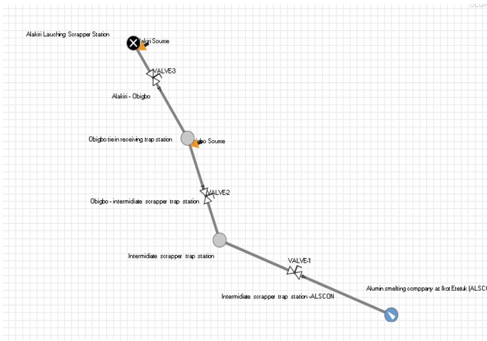
Figure 3. Schematic diagram of OLGA models with valves along the flow path with nodes and sources inlet
