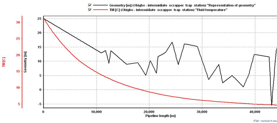
Figure 15. Temperature drop/variation along Obigbo-intermediate scrapper trap station within expected value
