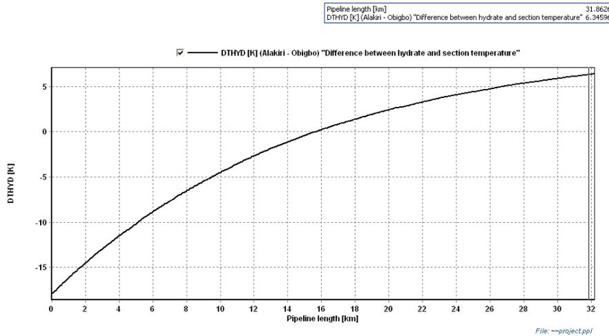
Figure 19. Alakiri – Obigbo different between Hydrate and section temperature
