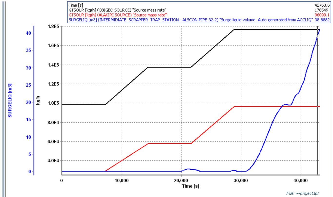
Figure 27. Alakiri Source and Obigbo mass rate and surge liquid volume for intermediate scrapper trap - ALSCON
