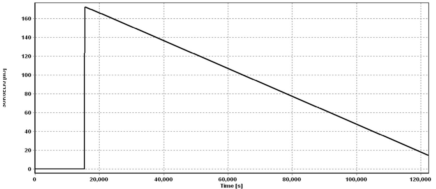
Figure 31. Plot of surge volume to determine the maximum pigging surge volume
