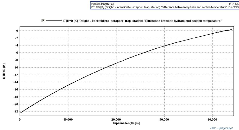
Figure 20. Obigbo - Intermediate scrapper Trapper station different between Hydrate and section temperature
