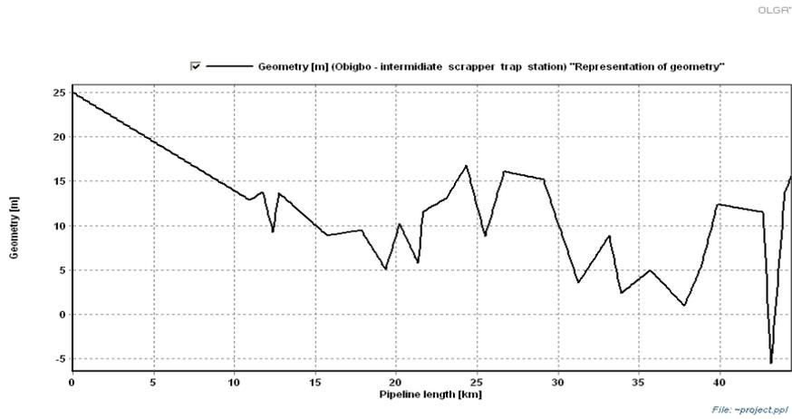
Figure 7. The Obigbo – Intermediate Scrapper Trap Station Profile Plots
