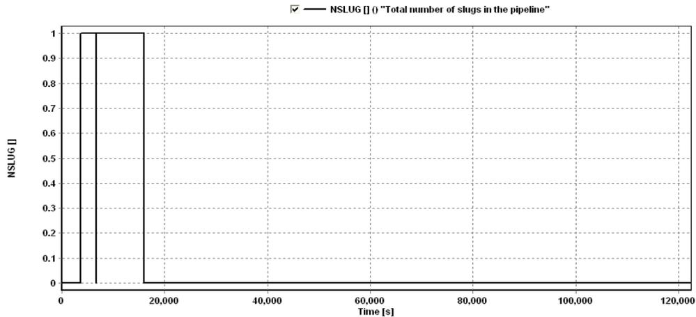
Figure 32. Plot of NSLUG to determine the total number of slugs in the pipeline
