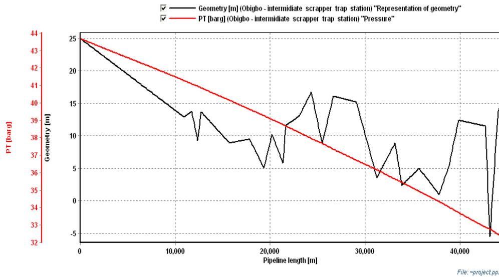
Figure 14. Pressure drop variation along Obigbo-intermediate scrapper trap station within expected value
