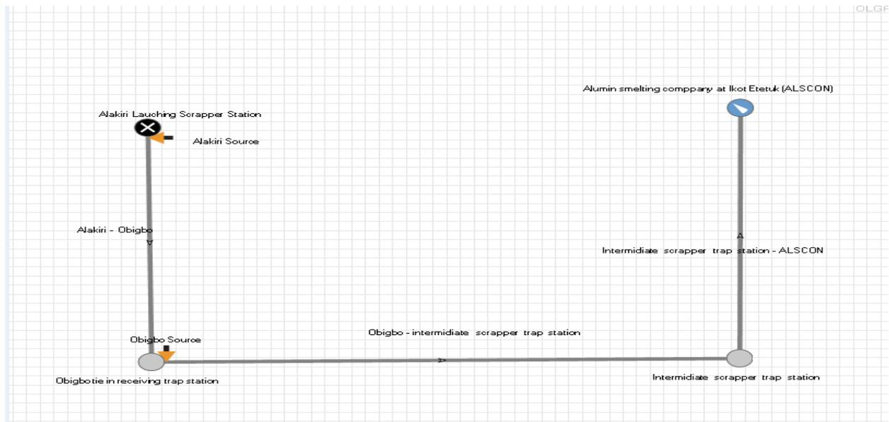
Figure 1. Schematic diagram of OLGA models with nodes and source inlet
