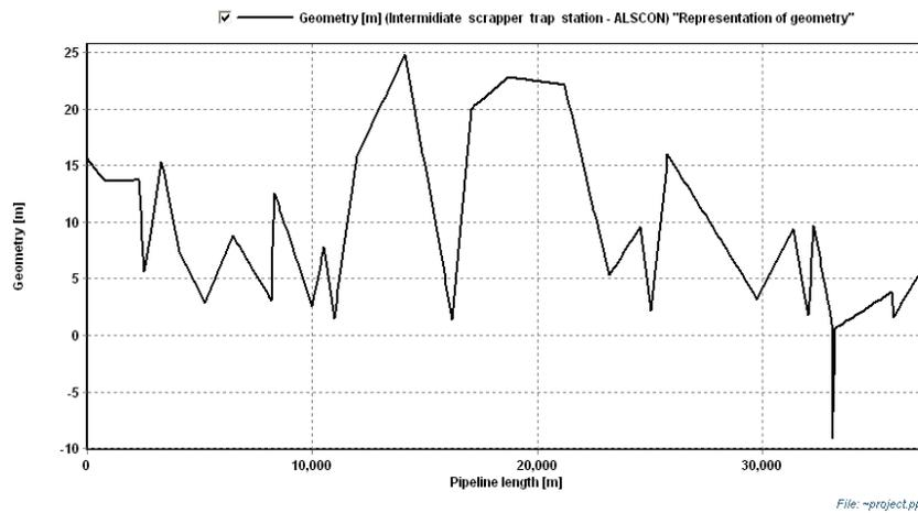
Figure 9. The Intermediate Scrapper Trap Station- ALSCON at Etetuk profile plots
