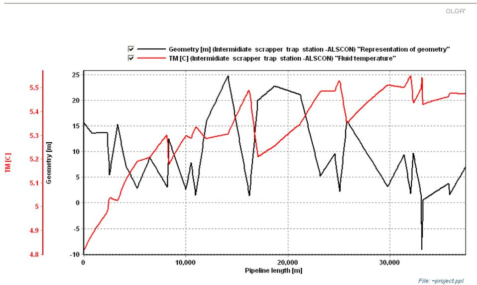
Figure 17. Temperature variation along intermediate scrapper trap-ALSCON less than expected value
