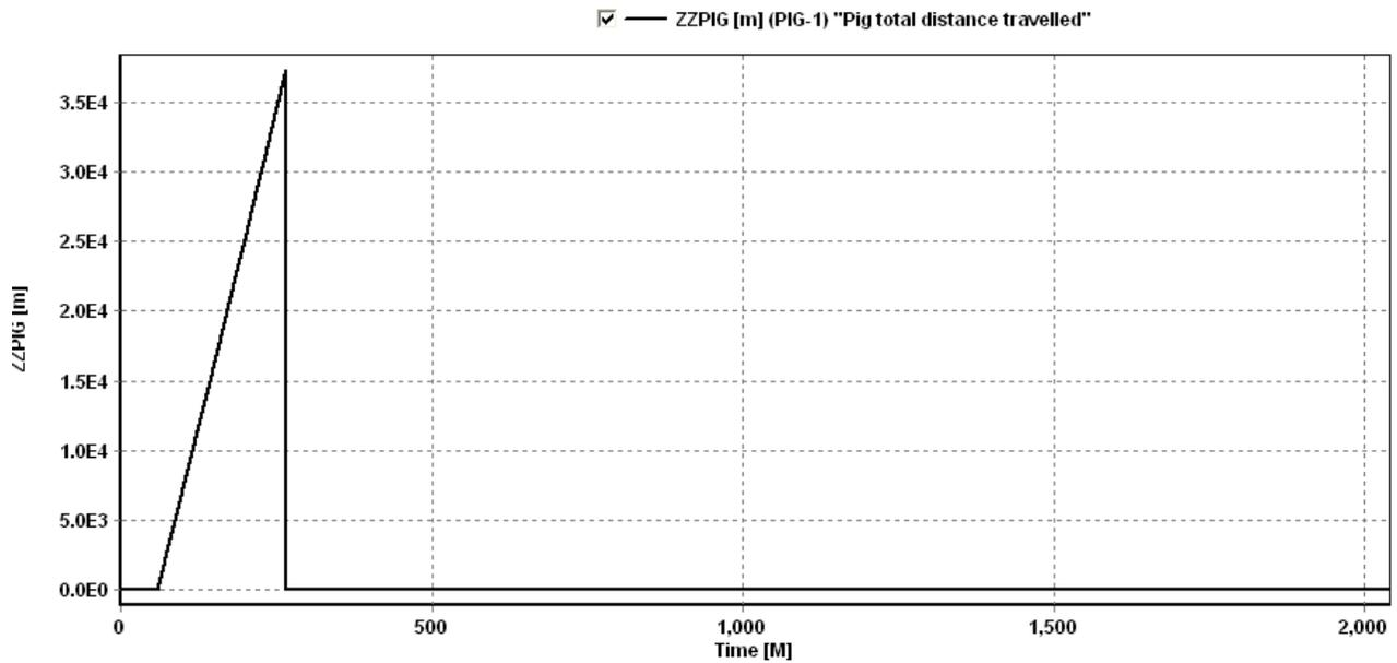
Figure 29. Pig trend plot of ZZPIG to determine when the pig reaches the trap
