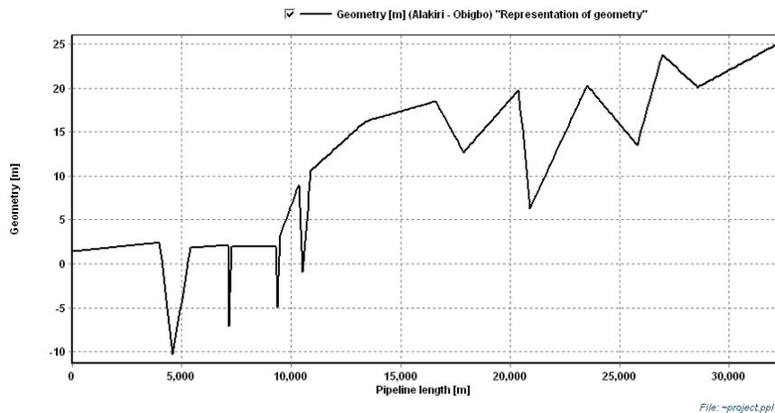
Figure 5. The Alakiri - Obigbo Trap Station Profile Plots
