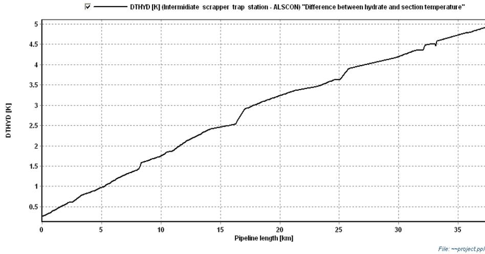
Figure 21. Intermediate scrapper trap station-ALSCON different between Hydrate and section temperature
