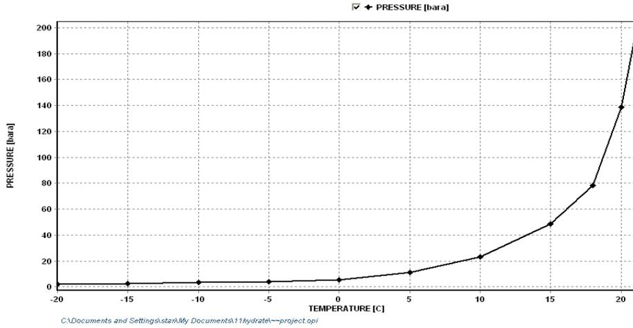
Figure 18. Hydrate curve
