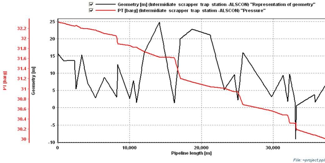
Figure 16. Pressure drop/variation along intermediate scrapper trap-ALSCON less than expected value
