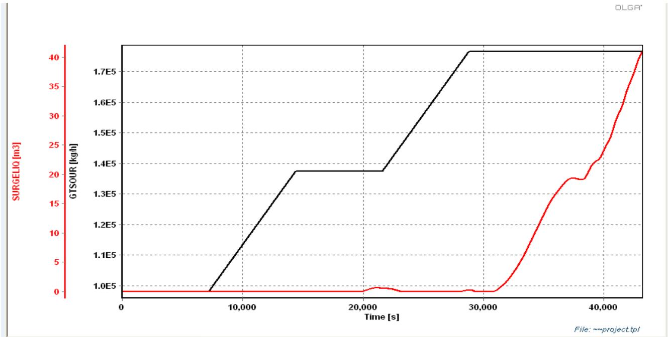
Figure 26. Obigbo Source mass rate and surge liquid volume for Intermediate scrapper trap - ALSCON
