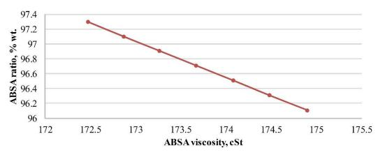
Figure 5. Dependence of ABSA mass ratio on its viscosity
