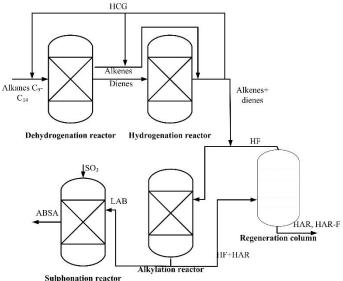
Figure 1. Flowchart of ABSA production: HCG - hydrogen-containing gas; HAR - high-aromatics; HAR-F - HAR fluorides
