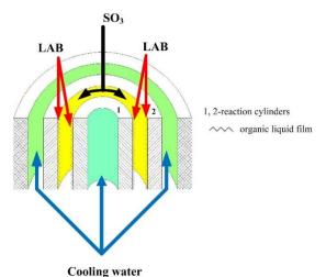
Figure 2. Design of sulphonation reactor
