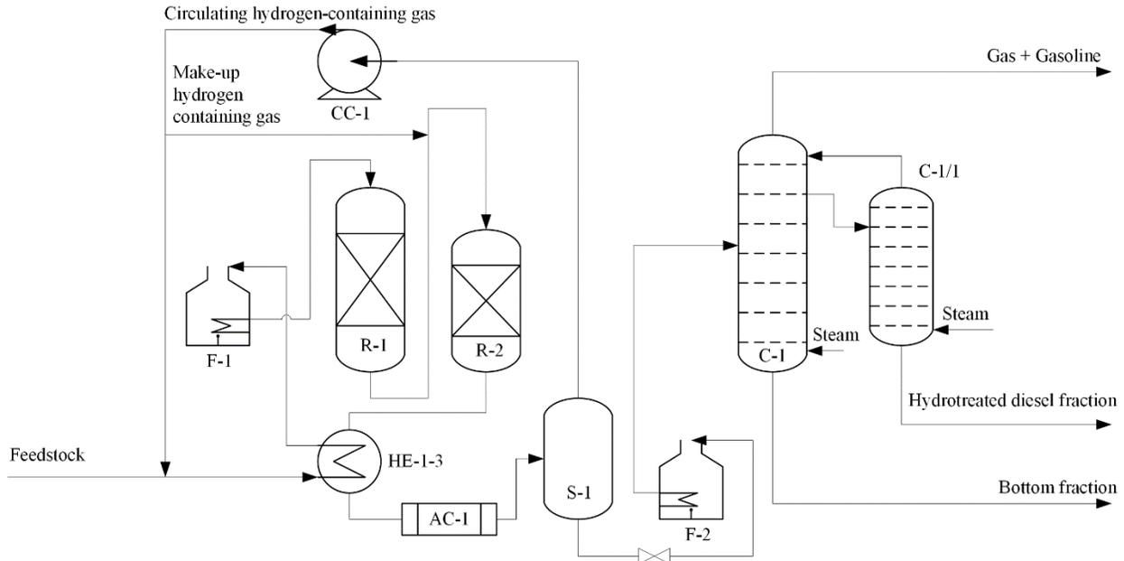
Figure 1. Process flow diagram of a combined unit for the production of low-sulfur diesel fuel with improved cold flow properties
