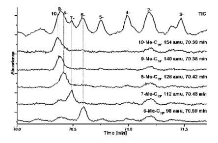
Fig. 6. Mass spectrometric deconvolution of GC unseparated isomers of monomethylnonadecanes in fuel diesel.
