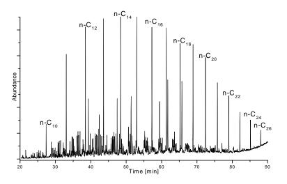
Fig. 5. GC-MS/TIC chromatogram of the separation of fuel diesel.
