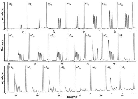
Fig. 1. Chromatogram of GC separation of  $C_9$ - $C_{30}$  monomethylalkanes with *n*-alkanes.
