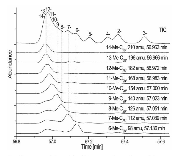
Fig. 2. Mass spectrometric deconvolution of GC unseparated isomers of monomethyloctacosanes.
