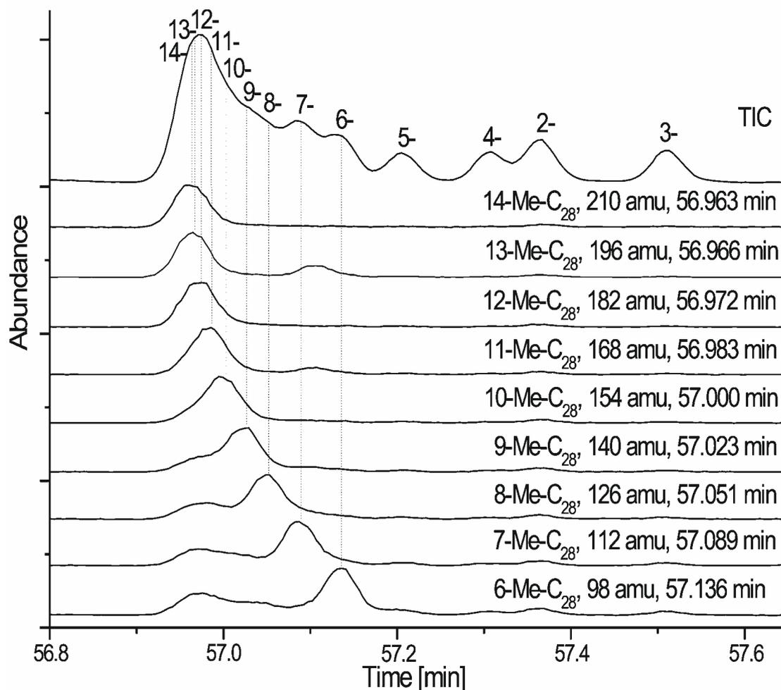
Fig. 2. Mass spectrometric deconvolution of GC unseparated isomers of monomethyloctacosanes.
