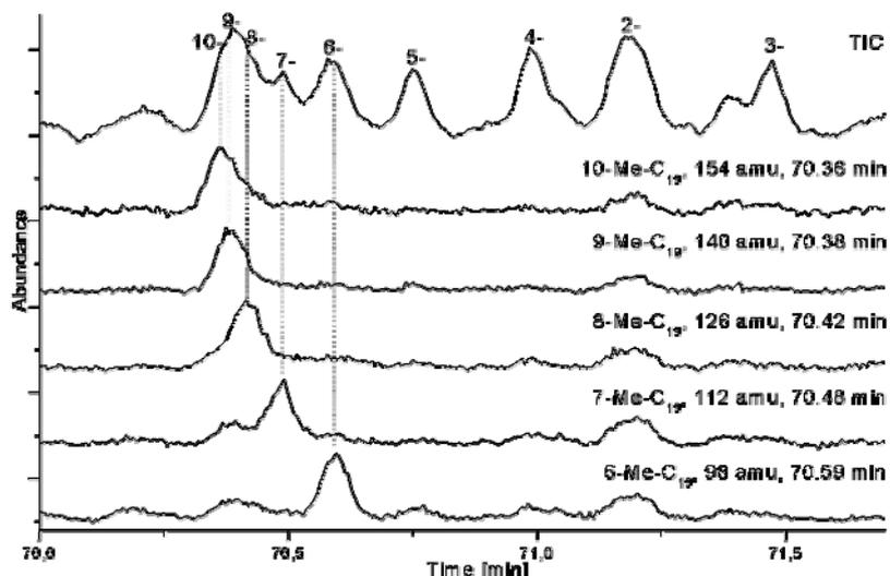
Fig. 6. Mass spectrometric deconvolution of GC unseparated isomers of monomethylnonadecanes in fuel diesel.
