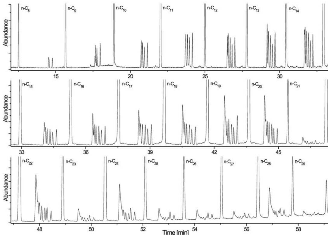
Fig. 1. Chromatogram of GC separation of C<sub>9</sub>–C<sub>30</sub> monomethylalkanes with *n*-alkanes.
