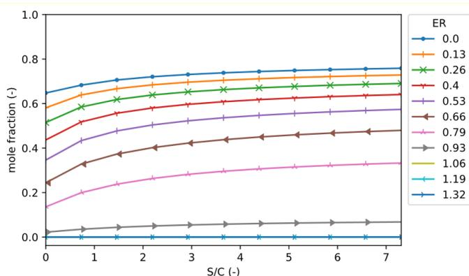
Figure 7. H<sub>2</sub> mole-fraction variation with S/C and ER
