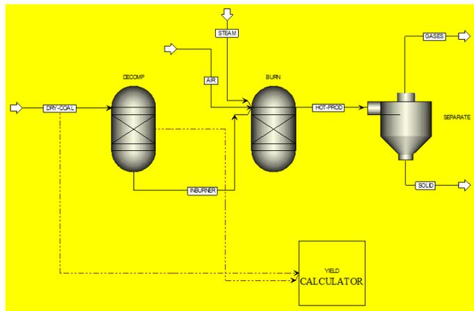
Figure 1. Flowsheet of lignite coal gasification in ASPEN
