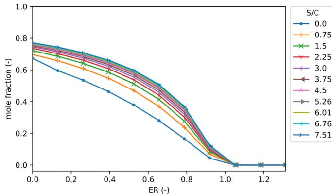
Figure 3. BMK H<sub>2</sub> Mole-fraction variation with ER and S/C
