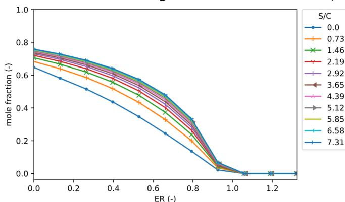
Figure 6. H<sub>2</sub> mole-fraction variation with ER and S/C
