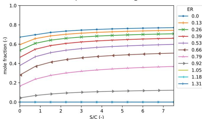
Figure 4. BMK H<sub>2</sub> Mole-fraction variation with SC and ER
