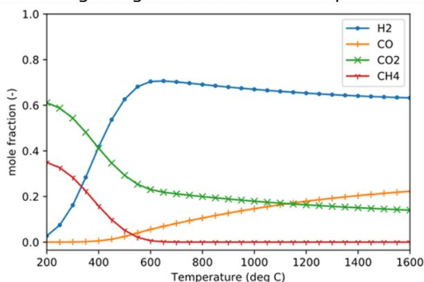
Figure 2. BMK product gas composition variation with temperature
