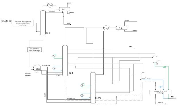
Fig. 3. The PFD equipped with an additional tray column, working in parallel with the main column K2 Alternatives of retrofit number 1, 2
