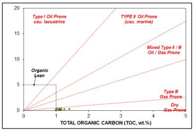
Fig. 6. Plot of S2 against TOC showing high level of thermal maturity of the organic matter and dry gas as the main hydrocarbon type
