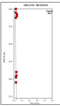
Figure 3. Plot of TOC against depth showing organic matter richness in studied section of Nzam-1 well
