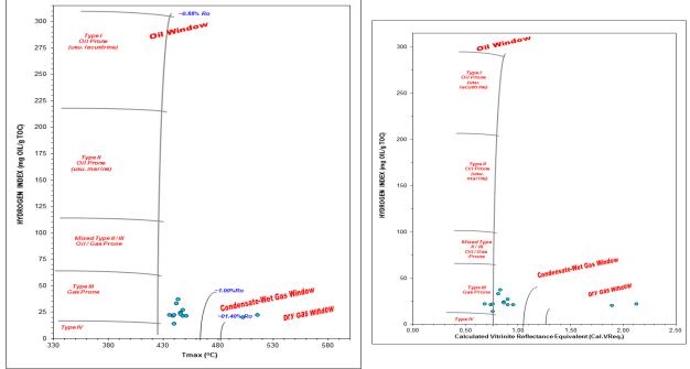
Fig. 4. Plot of Hydrogen Index against Tmax showing gas prone kerogen type III within the oil and condensate to wet gas windows
