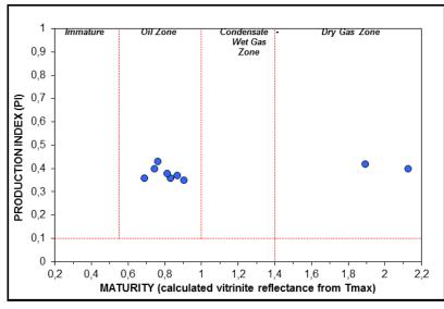
Fig. 7. Plot of Production Index against calculated vitrinite reflectance showing optimum maturity to post maturity of organic matter and oil with little dry gas zones
