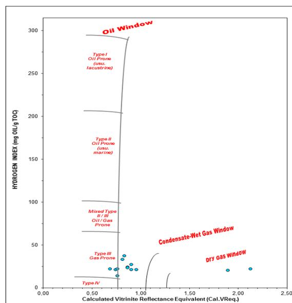
Fig.5. Plot of Hydrogen Index against Calculated Vitrinite Reflectance indicating gas prone kerogen type III organic matter within the oil window and dry gas windows
