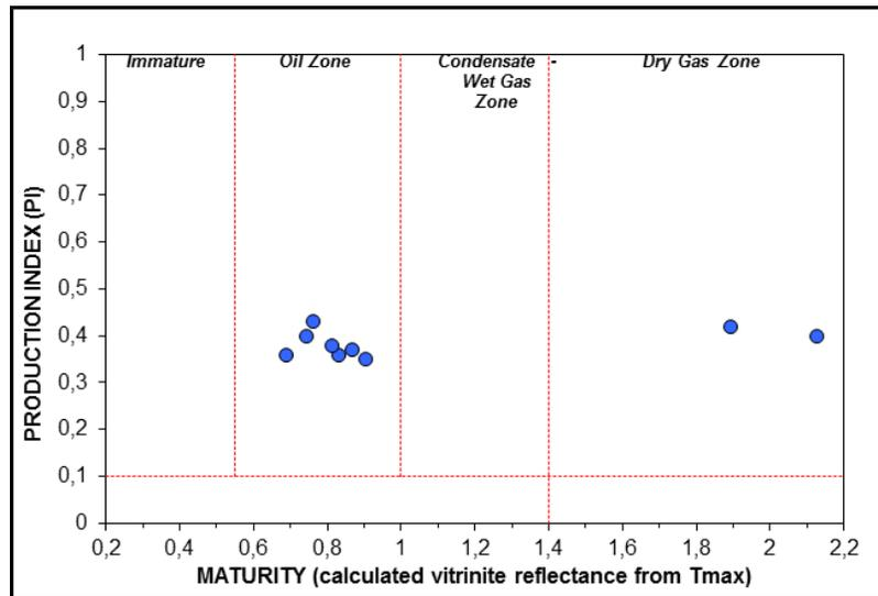
Fig. 7. Plot of Production Index against calculated vitrinite reflectance showing optimum maturity to post maturity of organic matter and oil with little dry gas zones
