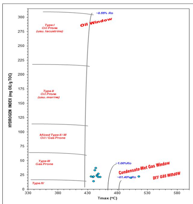
Fig. 4. Plot of Hydrogen Index against Tmax showing gas prone kerogen type III within the oil and condensate to wet gas windows
