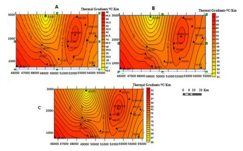
Fig. 7. Temperature fields at (a) 1000m, (b) 2000m and (c) 3000m
