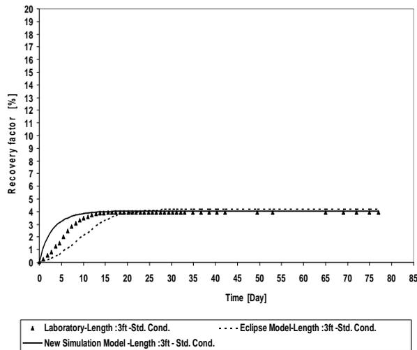
Figures 2 Variation of the oil recovery factor obtained after implementation of gravity drainage.
