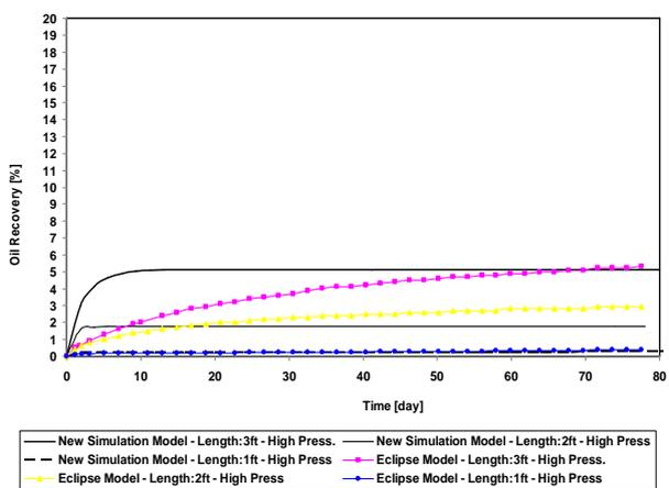
Figures 6 - Oil recovery factor versus time obtained after implementation of gas gravity drainage processes on the block scale at high pressure scenario (reservoir conditions) through Eclipse and proposed simulation model results.
