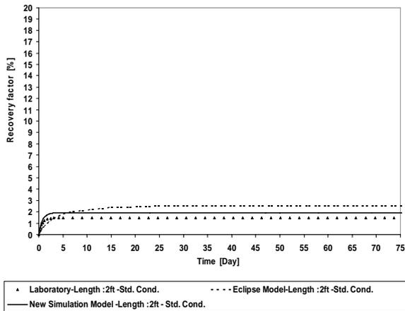
Figures 3 variation of the oil recovery factor obtained after implementation of gravity drainage
