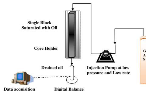
Figure 1 Schematic diagram for the gravity drainage process used in the experiments.
