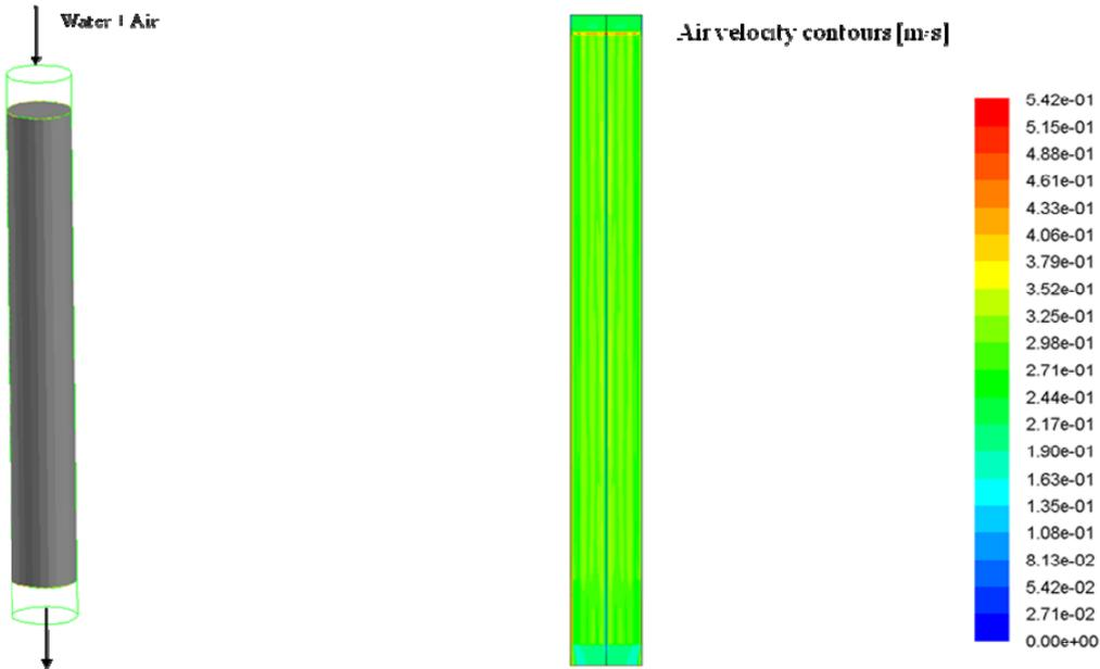
Fig.1. Contours of air velocity magnitude through porous media
