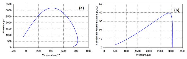
Fig. 1. Fluid data a) Phase envelope & b) Liquid dropout curve
