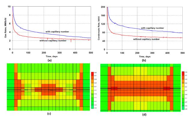
Fig. 5. Capillary number impact on a) Gas rate, b) Condensate rate. Plan view of condensate saturation around the fracture after 500 days c) without including capillary number & d) with including capillary number
