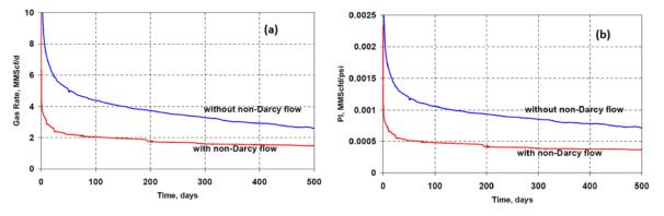
Fig. 4. Non-Darcy flow impact on a) Gas rate & b) Productivity index
