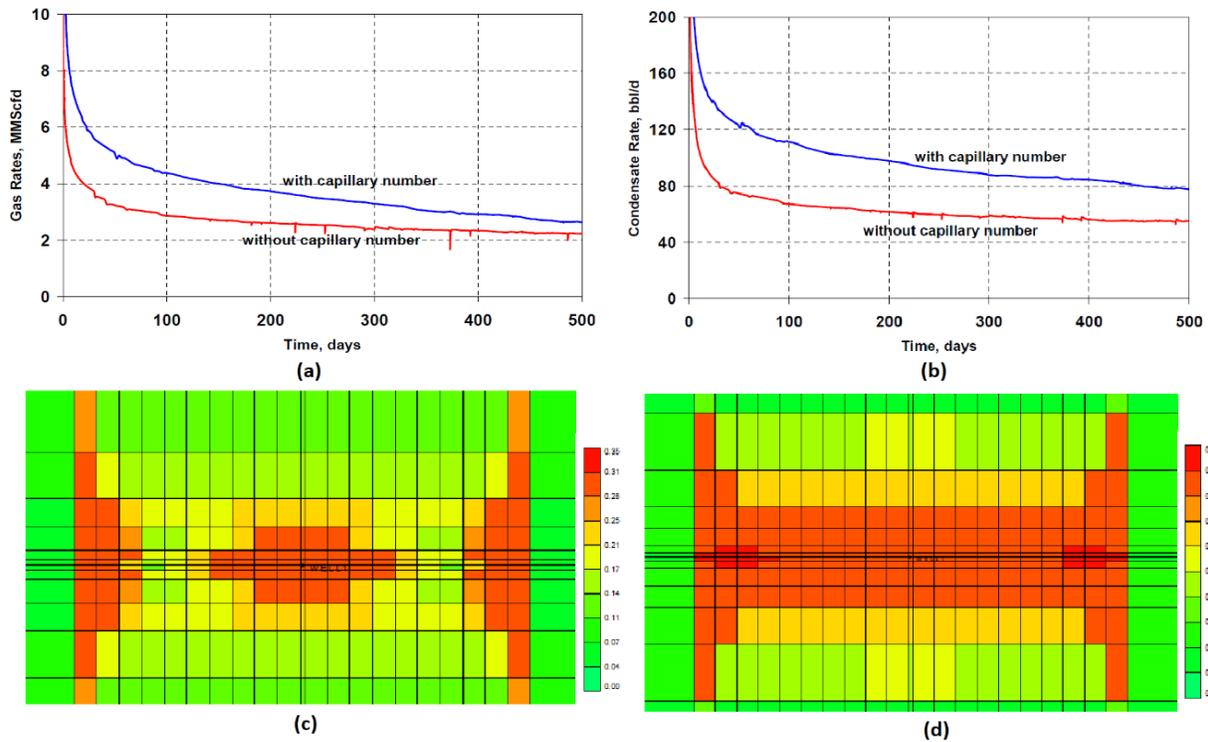
Fig. 5. Capillary number impact on a) Gas rate, b) Condensate rate. Plan view of condensate saturation around the fracture after 500 days c) without including capillary number & d) with including capillary number
