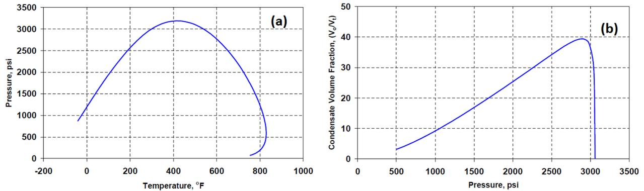
Fig. 1. Fluid data a) Phase envelope & b) Liquid dropout curve
