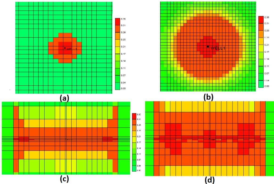
Fig. 3. Plan view of condensate saturation for a) “without fracture” after 800 days, b) “without fracture” after 3500 days, c) “with fracture” after 500 days & d) “with fracture” after 800 days
