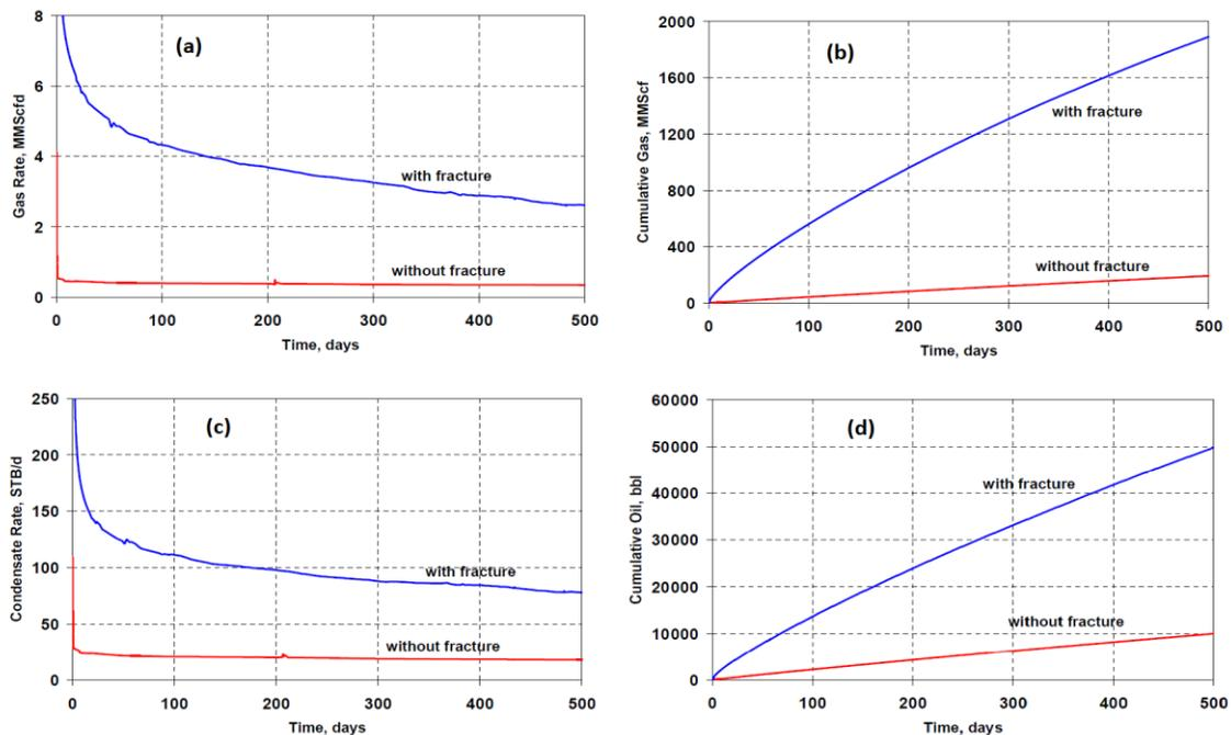
Fig. 2. Hydraulic fracture impact on a) Gas rate, b) Cumulative gas production, c) Condensate rate & d) Cumulative condensate production
