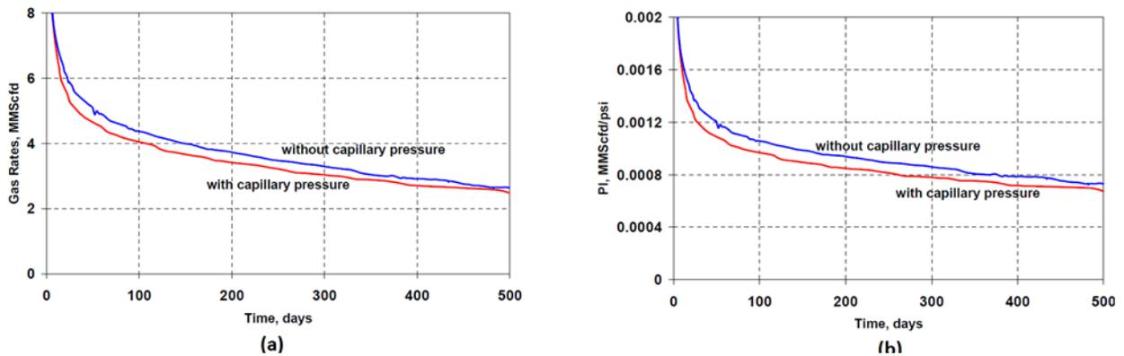
Fig. 6. Capillary pressure impact on a) Gas rate & b) Productivity index
