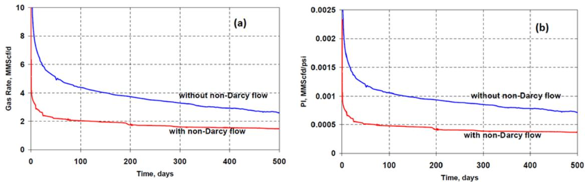
Fig. 4. Non-Darcy flow impact on a) Gas rate & b) Productivity index
