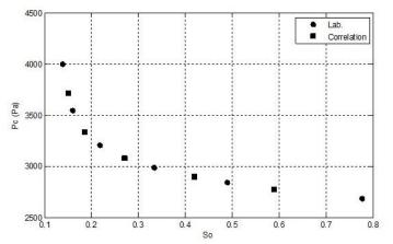
Figure 1 Comparative plot of observed and estimated values of capillary pressure during displacement period.
