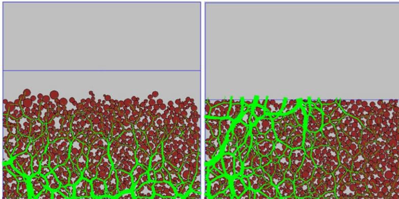
Fig.1. Contact forces between particles. Compression forces arising in coal batch under the action of gravity (left) and under the stamper impacts the coal cake (right) [13].
