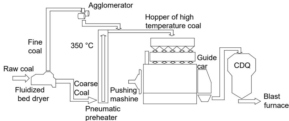
Fig. 4. Coke production technology, according to the SCOPE 21 project (modified after [21]).
