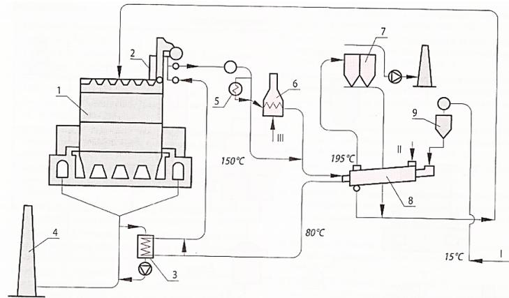
Fig. 2. Scheme of the installation for moisture control using CMC technology [9]:
