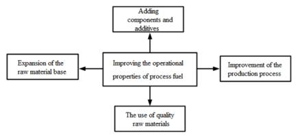
Figure 1. Block diagram showing the ways to improve the operational properties of process fuel
