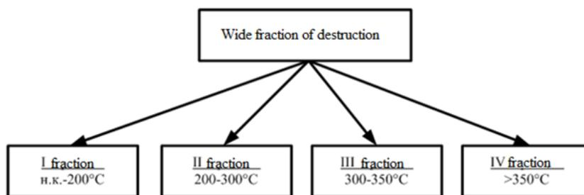
Figure .2 Products obtained by fractionation of a wide fraction thermal destruction
