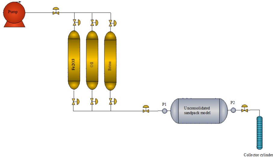
Figure 2. Schematic representation of displacement apparatus.
