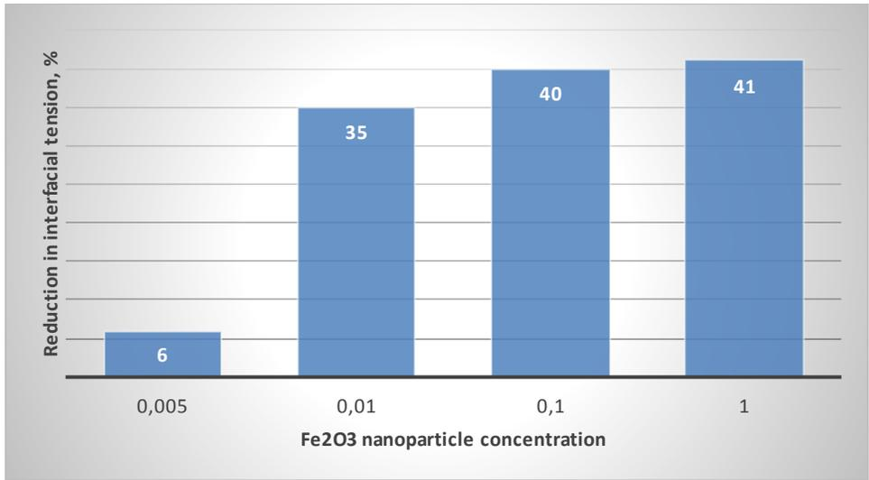
Figure 15. Effect of Fe<sub>2</sub>O<sub>3</sub> nanoparticle on interfacial tension
