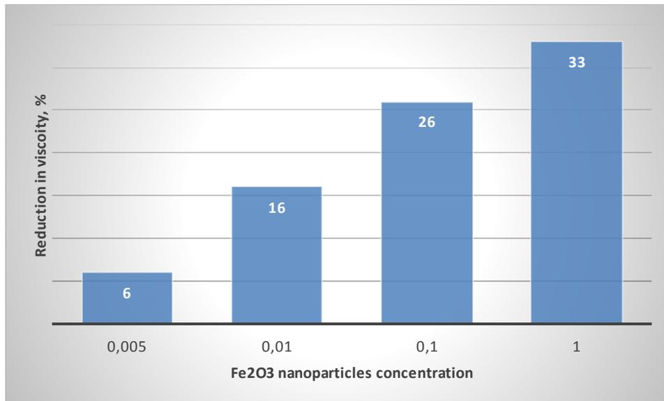
Figure 14. Effect of Fe<sub>2</sub>O<sub>3</sub> nanoparticle on crude oil viscosity
