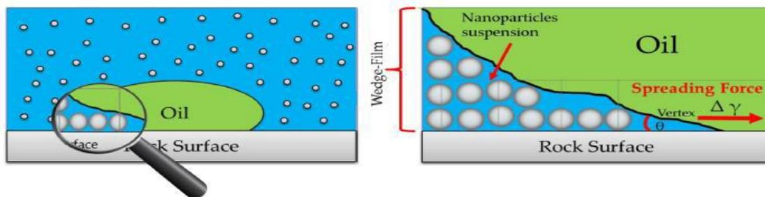
Fig. 1. Clarifying the joint mechanism due to the presence of nanoparticles in the injection fluid
