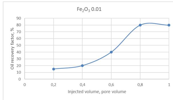
Fig. 7. Relative permeability curve at 0.01 wt %  $Fe_2O_3$  Fig. 8. Effect of 0.01 wt %  $Fe_2O_3$  on oil recovery
