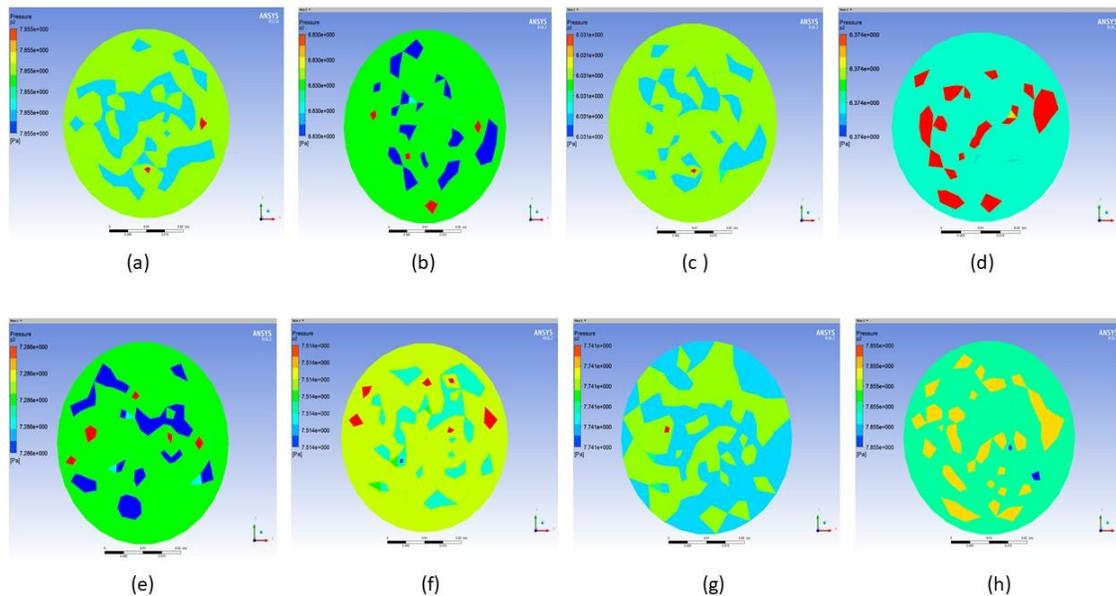
Figure 10. Pressure contours at a position of  $Z=2\text{m}$  for a) crude oil, b) crude oil+50 mg/L of NS, c) crude oil+100 mg/L of NS, d) crude oil+150 mg/L of NS, e) crude oil+200 mg/L of NS, f) crude oil+300 mg/L of NS, g) crude oil+500 mg/L of NS, h) crude oil+700 mg/L of NS
