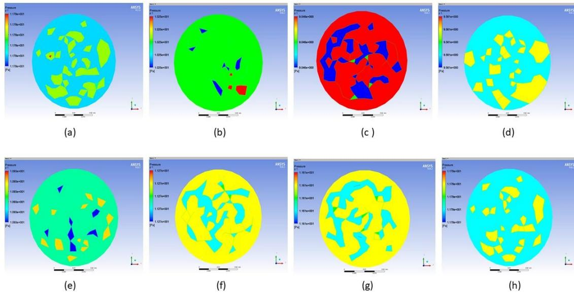
Figure 9. Pressure contours at a position of  $Z=1\text{m}$  for a) crude oil, b) crude oil+50 mg/L of NS, c) crude oil+100 mg/L of NS, d) crude oil+150 mg/L of NS, e) crude oil+200 mg/L of NS, f) crude oil+300 mg/L of NS, g) crude oil+500 mg/L of NS, h) crude oil+700 mg/L of NS
