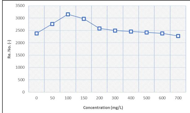
Figure 5. Reynolds number values as a function of NS concentration
