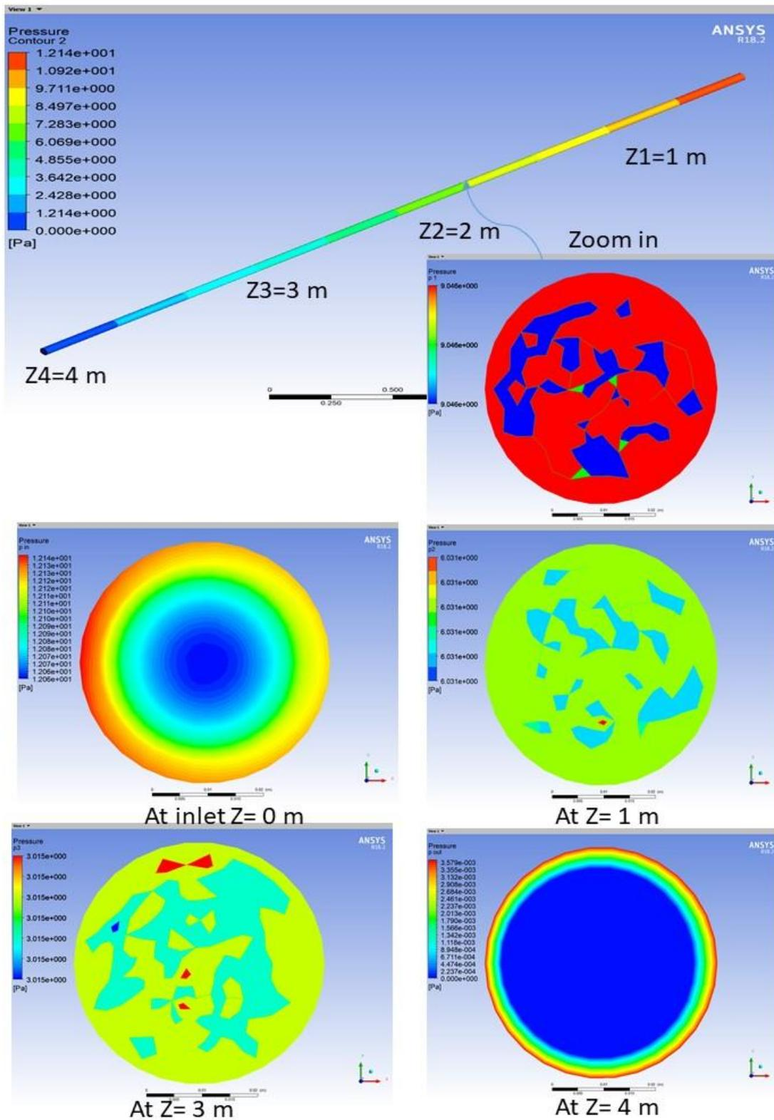
Figure 8. Pressure contours for the crude oil with optimum NS concentration
