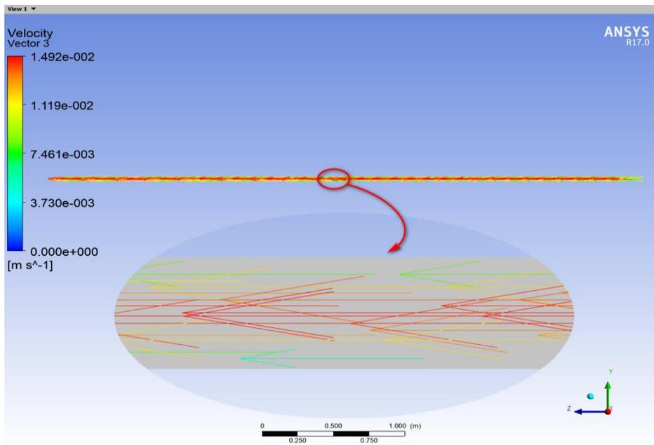
Figure 13. Velocity contour of the crude oil sample inside the pipe at different positions
