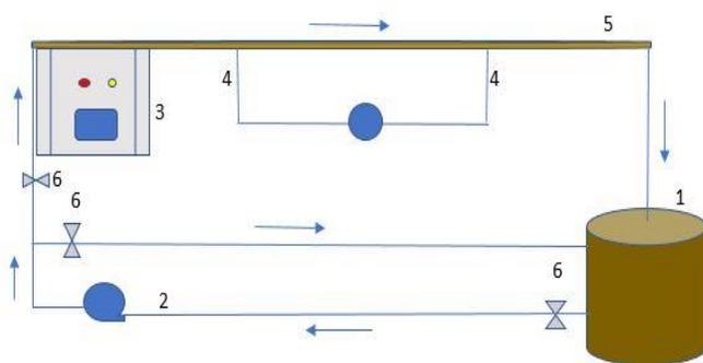
1- Tank, 2- Pump, 3- Control unit, 4- Pressure transducer, 5- Pipe, 6- Valve.
