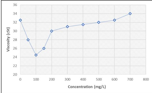
Figure 4. Effect of NS concentration on crude oil viscosity
