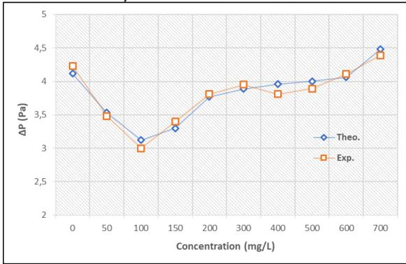
Figure 6. Effect of NS concentration on differential pressure
