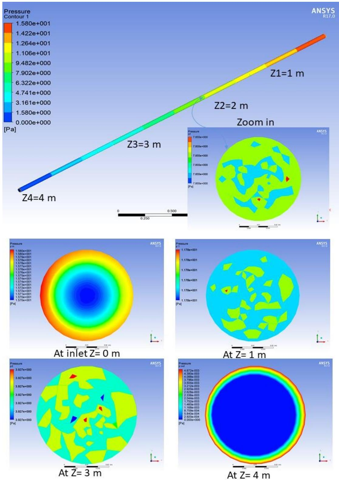
Figure 7. Pressure contours for the crude oil without NS
