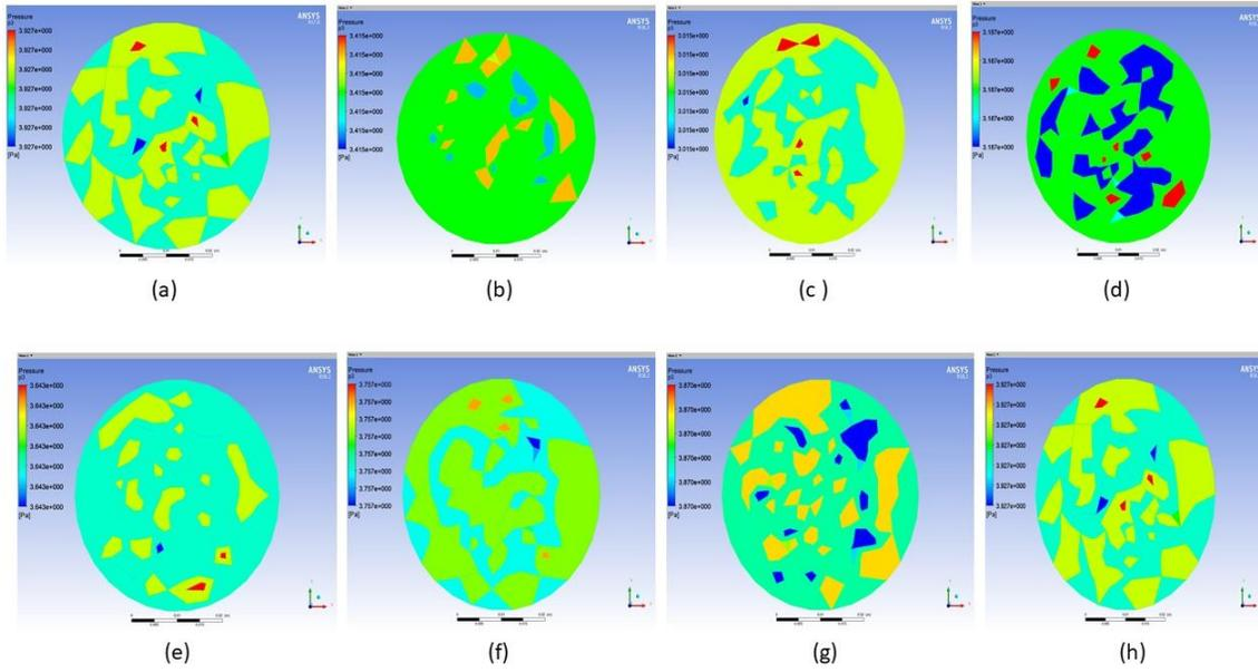
Figure 11. Pressure contours at a position of Z=3m for a) crude oil, b) crude oil+50 mg/L of NS, c) crude oil+100 mg/L of NS, d) crude oil+150 mg/L of NS, e) crude oil+200 mg/L of NS, f) crude oil+300 mg/L of NS, g) crude oil+500 mg/L of NS, h) crude oil+700 mg/L of NS
