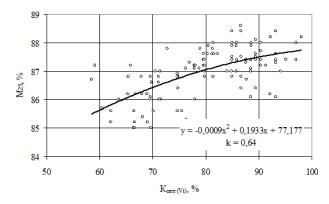
Fig. 1. Dependence of coke strength  $M_{25}$  on  $K_{opt(Vt)}$
