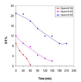
Fig. 5 Effect of molecular weight on degradation of Oppanol B additives, at Q = 6 m<sup>3</sup>/hr, 50 ppm concentration and 31.75 mm I.D
