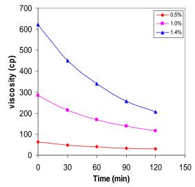
Fig. 4 Concentration effect on viscosity for Oppanol B-250 solution at 1800 rpm
