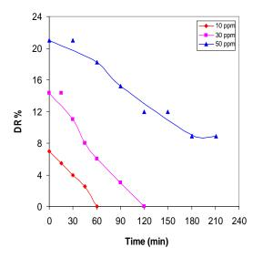
Fig. 6Time dependence of percentage drag-reduction for Oppanol B 250 at different concentration, 6 m<sup>3</sup>/hr flow rate and 31.75 mm I.D
