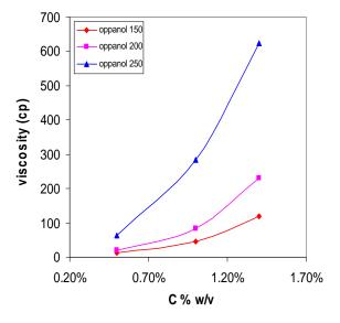
Fig. 2 Combined effect of concentrations and molecular weight on the viscosity of Oppanol B solutions
