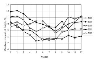
Fig.2. Variation in the moisture content of coal batch at coke batteries 1–4 between 2008 and 2012  $\,$
