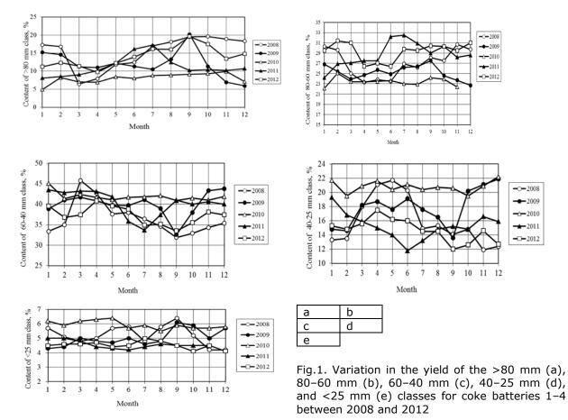
In studying the influence of the moisture content on the size distribution of the coke, we find that for from 11.9% in January 2009 to 9.5% in August 2009 (Fig. 2) is accompanied by decrease in the yield of the >80 mm class from 15.2 to 13.3% and in the yield of the 80–60 mm class from 27 to 26.4%. There is no significant change in the yield of the 60–40 mm class.
