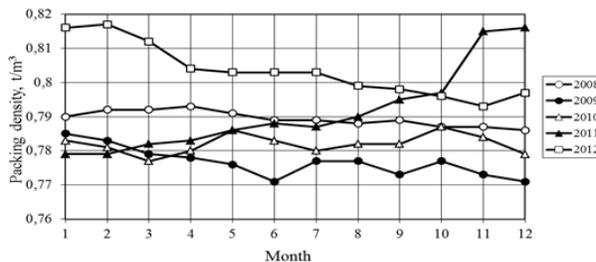
Fig.5. Variation in the packing density of the coal batch at coke batteries 1–4 between 2008 and 2012
