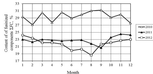
Fig.6. Variation in the content of fusinized components ( $\Sigma FC$ ) in the coal batch at coke batteries 1–4 between 2010 and 2012
