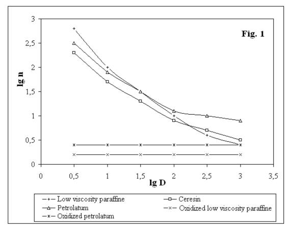
Figure 1. Dependence of logarithm of gradient of velocity of deformation (lg D) from logarithm of viscosity (lg n) of FAOC with different thickeners.
