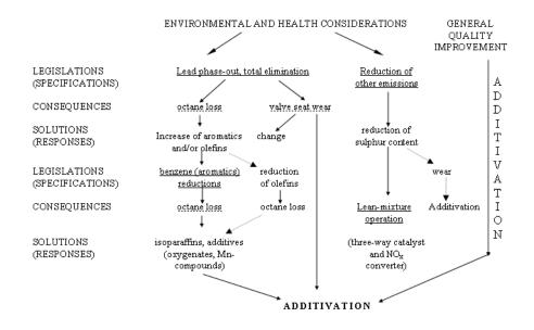
Figure 2. An example of causes and trends of quality changes in engine gasolines
