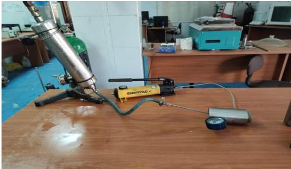
Figure 2. Core holder displacement system
