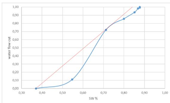
Figure 13. Fractional flow curve for 0.01 alumina flooding
