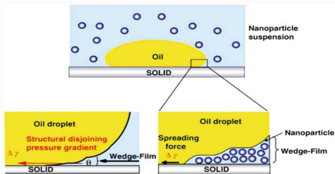
Figure 1 Nanoparticles creates wedge-film structure
