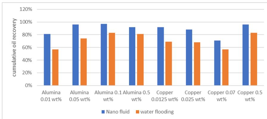
Figure 6. Water flooding VS Nano flooding
