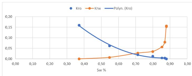
Figure 4. Relative permeability curve for 0.01 wt% alumina flooding
