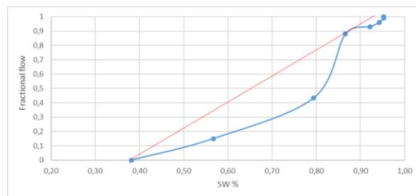
Figure 14. Fractional flow curve of 0.0125 wt% copper at core S56
