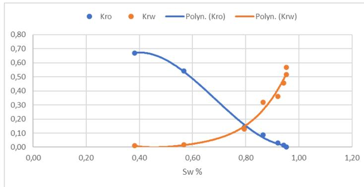
Figure 5. Relative permeability curves at 0.0125 wt% copper oxide
