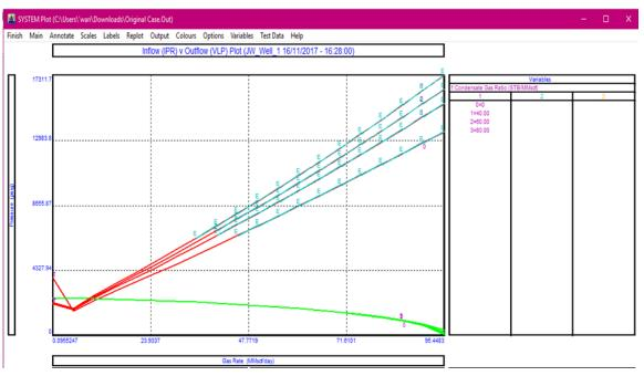
Fig. 7. VLP/IPR matching showing various CGR
