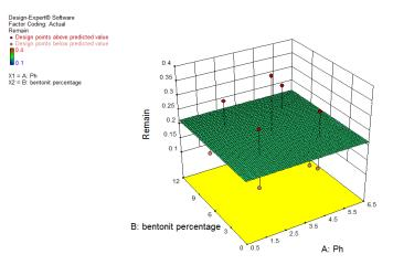
Fig. 6. The plot related to the remained percentages on the sieve 850  $\mu m$  in terms of bentonite percentage and pH
