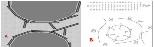
Fig. 1. A photomicrograph of a bitumen emulsion stabilized with (a) clay particles, (b) chemical emulsifier <sup>[5-6]</sup>
