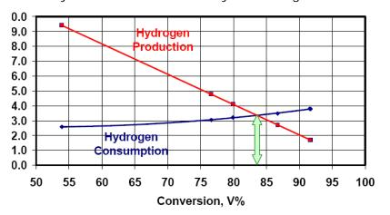
Figure 3 Hydrogen balance point <sup>[14]</sup>
