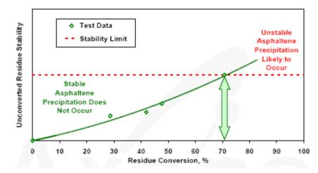
Figure 2 Stability Limit for ebullated bed hydrocracking conversion level <sup>[14]</sup>
