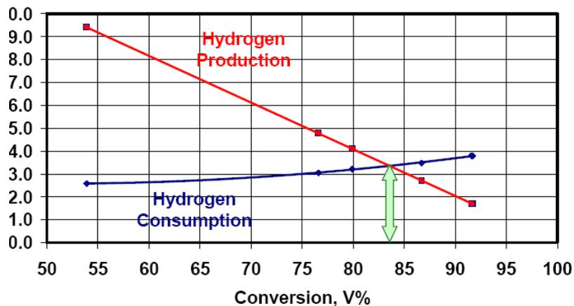
Figure 3 Hydrogen balance point [14]
