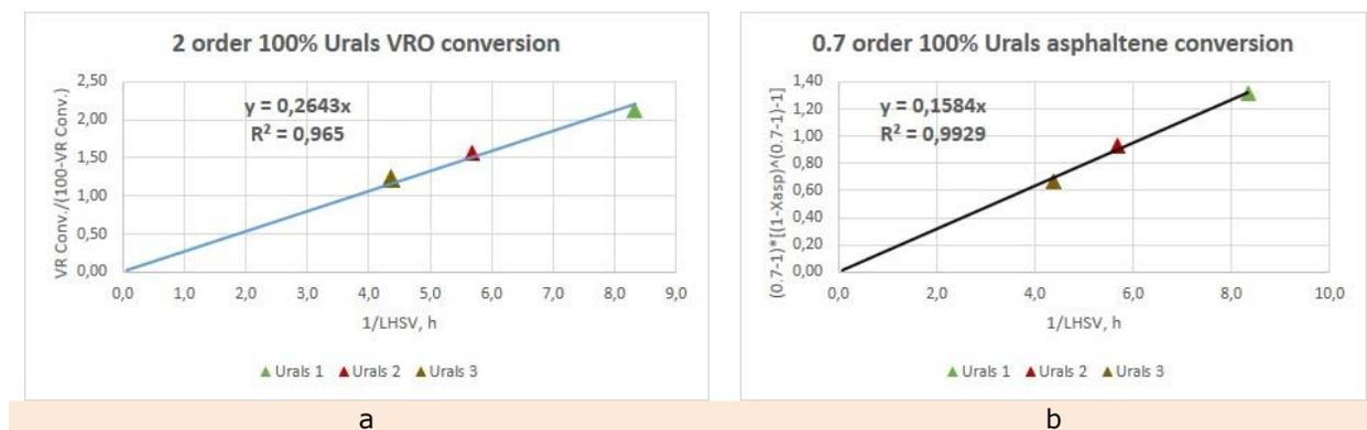
Figure 3. Second order kinetic plot for the 100% Urals VRO conversion (a) and 0.7 order kinetic plot for the 100% Urals asphaltene conversion at a reaction temperature of 410°C (b)
