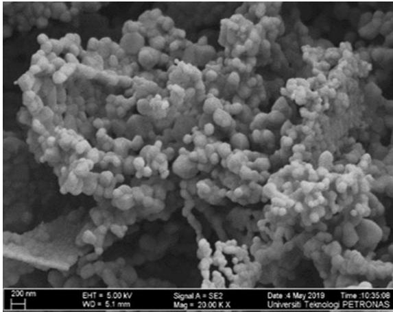
Fig. 4. FESEM image of zinc oxide nanoparticles
