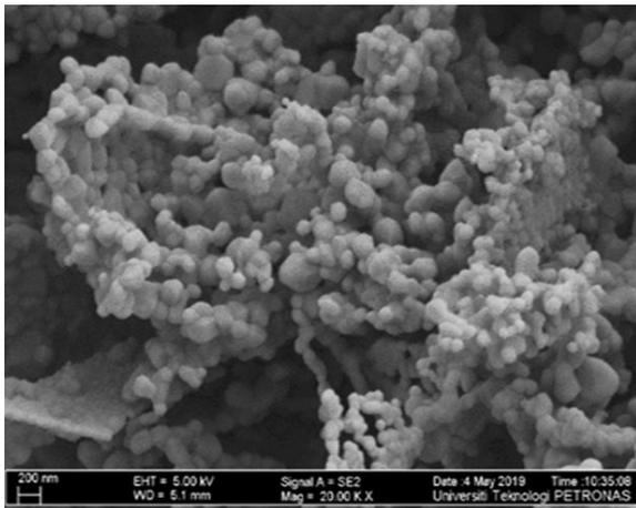
Fig. 4. FESEM image of zinc oxide nanoparticles
