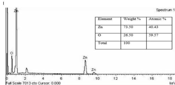
Fig.5. EDX result showing elements composition and distribution
