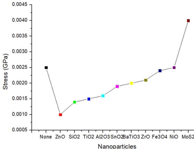
Fig. 3. Graphical result of surface stress obtained between oil/rock interface with and without NPs
