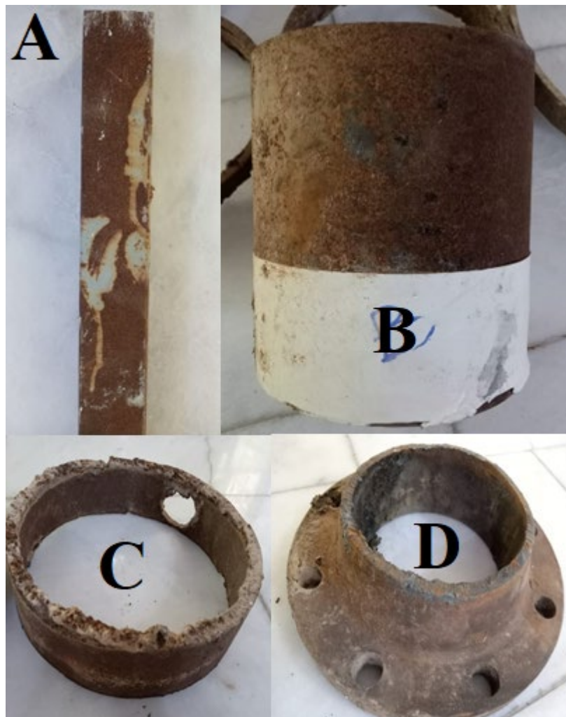
Figure 2. Oil pipelines samples. (A) Ductile Iron, (B) X60 Carbon Steel, (C) X80 Carbon Steel, (D) A 105 for pipe.
